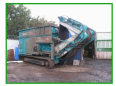
When they finally cool down they are left to stabilize. The whole process takes 16 weeks. Eventually they are screened at different meshes to give soil improvers, biofuel and topsoil, and these are sold.
